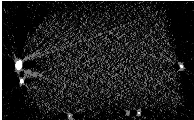
Fig. 6. DART reconstruction of a slice of the Catalyst dataset in the xz -plane. The brightness of the support material was increased for clarity.
