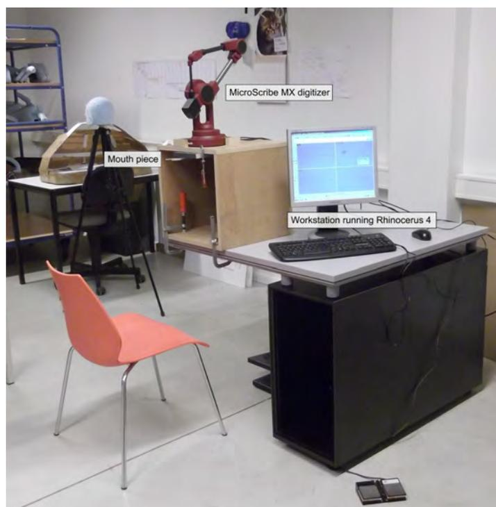
Figure 43: Experiment setup. The test subject was seated on the red chair, biting down on the white mouth piece to stabilize their head. The box fixating the MicroScribe was positioned such that the experimenter could comfortably move the digitizer's arm around the person's head.
