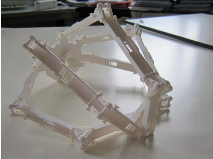
Figure 5: OpenBCIs second 3D-printed "SpiderClaw" headset prototype.
