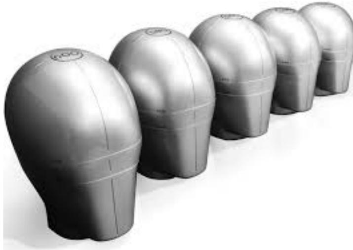
Figure 19: Example of a set of EN960 headforms (manikins). Image from "SizeChina: 3D anthropometric survey of the Chinese head" [50].
