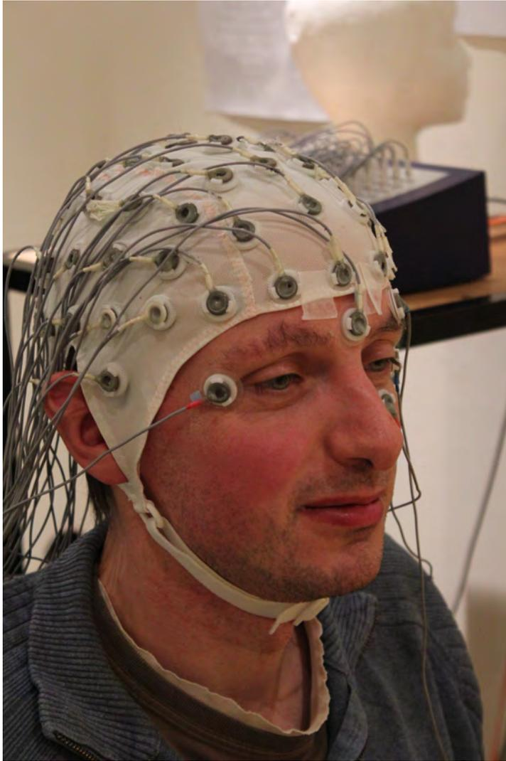
Figure 3: EEG cap with gel-based electrodes inserted. Photo by Chris Hope, made available by Tim Sheerman-Chase at [29] through CC BY 2.0 license [30]
