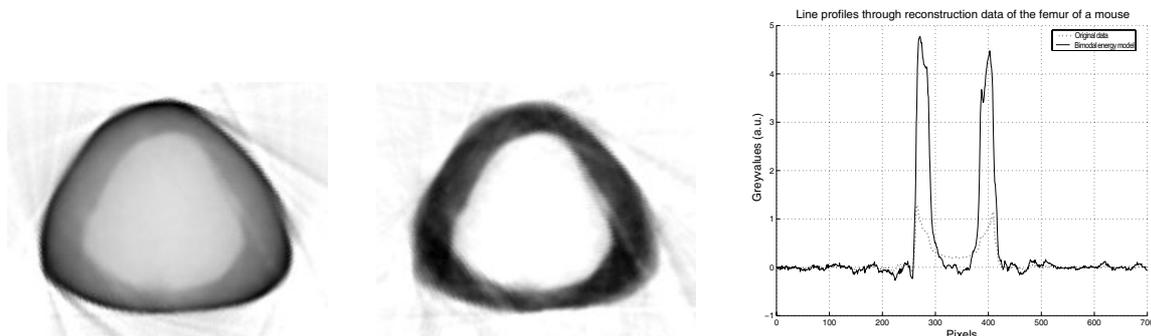
**Figure 8.** The attenuation profiles (right) and reconstructed images of a bone, before (left) and after (middle) beam hardening correction. Note that the greyvalues in the reconstructed images are scaled between zero and their maximum value.
