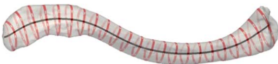
Fig. 2. Visualization of some (23) circumferential lines of the parameterization on the cylinder together with the CL that connects the centers of the circumferential lines.
