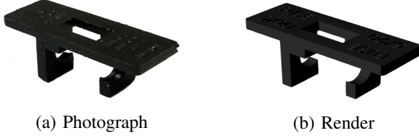
Fig. 3. The fuse cover sample: (a) shows a photograph of the real sample and (b) shows a render of the CAD model.
