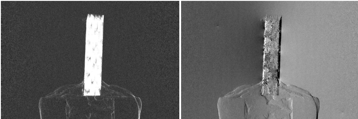
Figure 5: Actual DFC (left) and DPC (right) images of a CFRP. The DFC image has been log-corrected, such that a stronger dark field signal corresponds to a higher grey value. Images were acquired with a Bruker SkyScan 1294 phase contrast micro-CT system.
