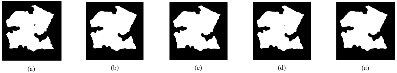
Figure 5: (a) The phantom, (b) segmented THz-SIRT reconstruction at 200 iterations, (c) THz-DART reconstruction for P = 1 after 500 iterations, (d) THz-DART reconstruction for P = 0.7 after 500 iterations, (e) segmented THz-SIRT reconstruction after 500 iterations.
