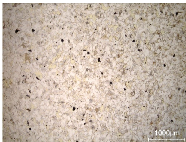
Fig. 15 Photomicrograph showing the general appearance of Obernkirchen sandstone under a polarizing microscope (single polarized light). The intergranular pores are visible in yellow on the picture. Quartz grains (nonporous) appear white. Rock fragments (microporous) appear in light grey.
