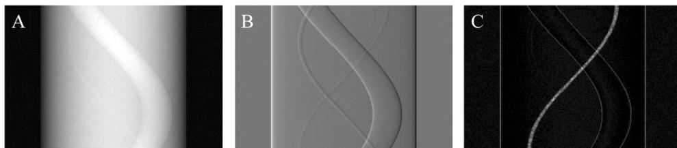
**Fig. 12.** Simulated sinograms for A) absorption contrast; B) differential phase contrast; and C) dark field contrast.
