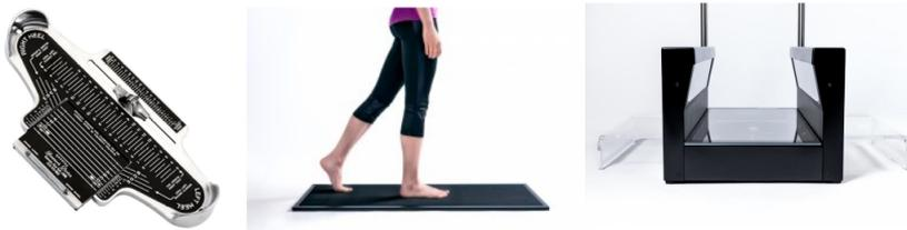
Figure 1.3: **Some measurement equipment used to evaluate foot shape.** From left to right: Brannock device, plantar pressure plate, 3D laser scanner.
