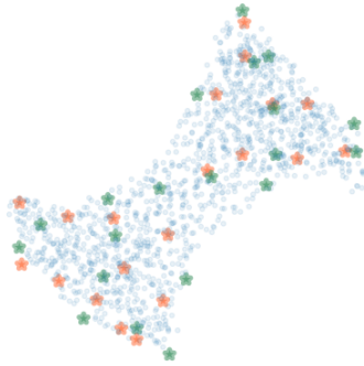
Fig. 4.7 The bounding (green) and SIFT (orange) landmarks of a bone with random bone voxels in blue. The landmarks are distinguishable and at a distinctive distance from each other.
