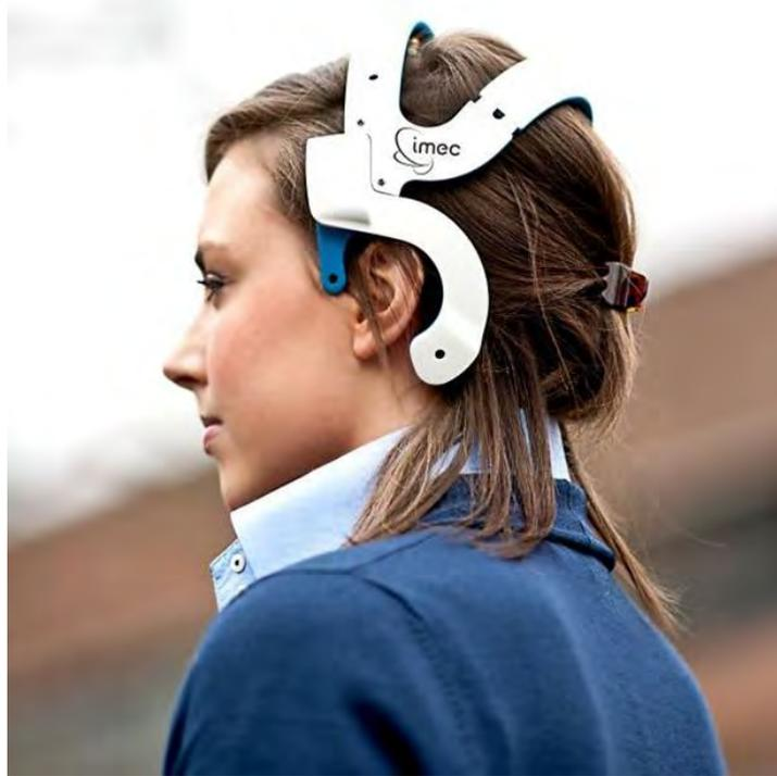
Figure 6: A prototype BCI headset with dry electrodes, created by Imec for research purposes. Image from NeuroGadget [40].
