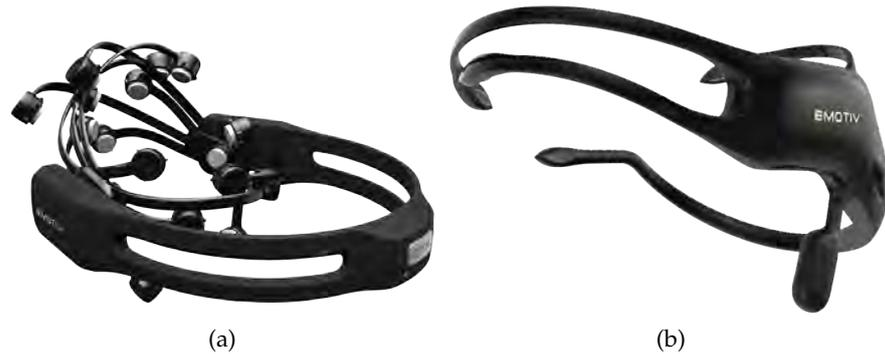
Figure 4: Emotiv’s research-grade Epoc+ headset (a) and consumer-grade Insight headset (b). Both images were made available by Wikimedia user Chrisshe at [35] (a) and [36] (b) through the CC BY-SA 4.0 license [37].
