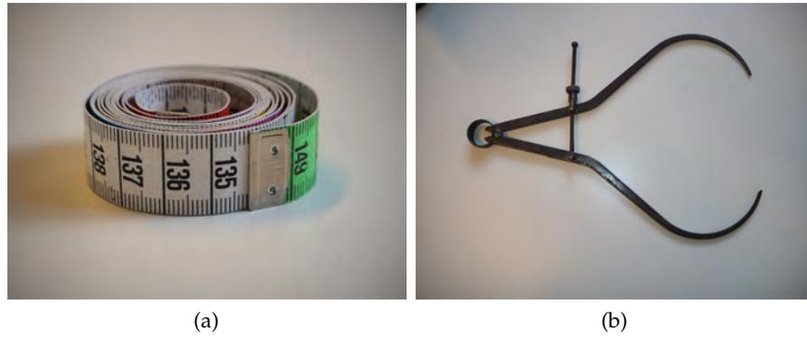
Figure 11: Common anthropometric tools: a tape measure (a) and outside calipers (b).
