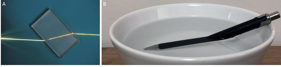
Figure 2.1: (a) A ray of visible light refracting at the air-material boundaries of a transparent piece of plastic. (b) Distorted view of a pen partially submerged in water due to refraction of light.
