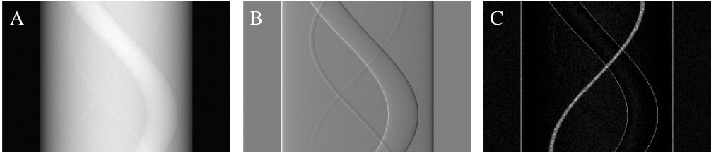
Figure 3.10: Simulated sinograms for (a) absorption contrast; (b) differential phase contrast; and (c) dark field contrast. Color scale bars are omitted due to the qualitative nature of the discussion in the main text.
