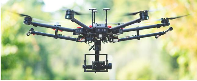
**Fig. 1.** The dual hyperspectral snapshot UAV payload mounted on a DJI M600 pro.
