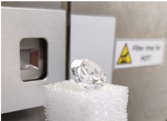
Figure 3: the 7-carat diamond in front of the X-ray source of the CT scanner.
